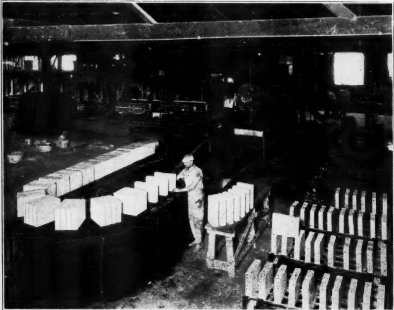
Automatic Machine Making 3 Inch Partition Tile
